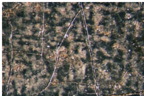
Fig. 4.9.2 The oil residues manifest either as blanchy material ( left ) or as crusty orangey material ( right ).
