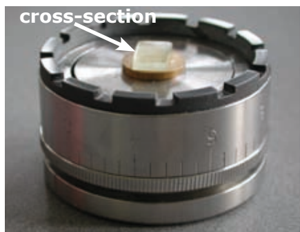
Fig. 1.1 Adjustable polishing holder.
